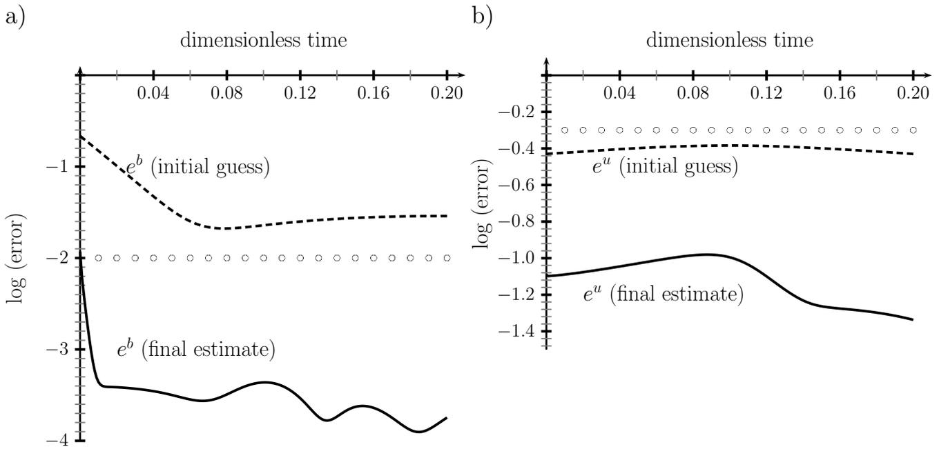
**Fig. 5.** Dynamical evolution of  $L_2$  errors (logarithmic value) for the magnetic field (a) and the fluid velocity (b). Dashed lines: errors for initial guesses. Solid lines: errors after variational assimilation. Circles represent instants where magnetic observations are made. In this particular case,  $nt=20$  and  $n^S=20$ .
