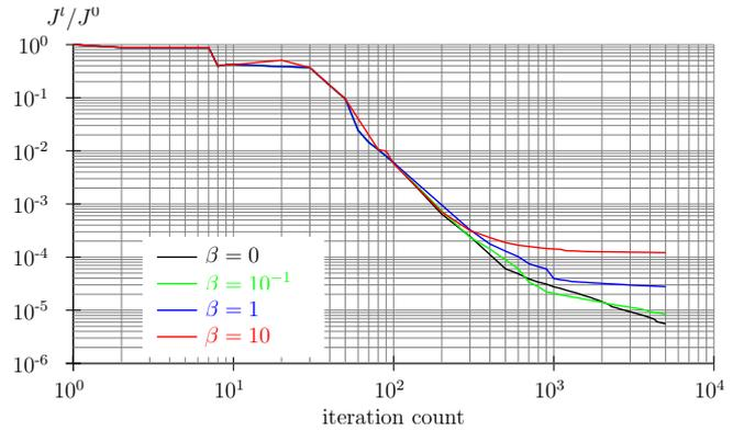
**Fig. 10.** Convergence behaviour for different constraint levels  $\beta$ . The ratio of the current value of the misfit  $J^l$  (normalized by its initial value  $J^0$ ) is plotted against the iteration count  $l$ .  $\beta$  measures the strength of the constraint imposed on the state relative to the observations.
