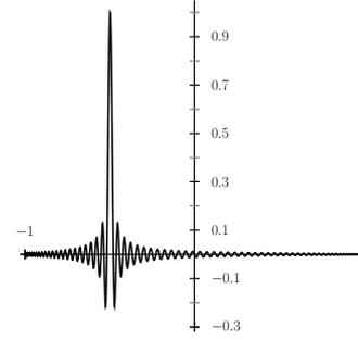
**Fig. 1.** An example of a basis function used to discretize the MHD model in space. This particular Lagrangian interpolant,  $h_{50}^{150}$ , is obtained for a polynomial order  $N=150$ , and it is attached to the 51st Gauss–Lobatto–Legendre point.
