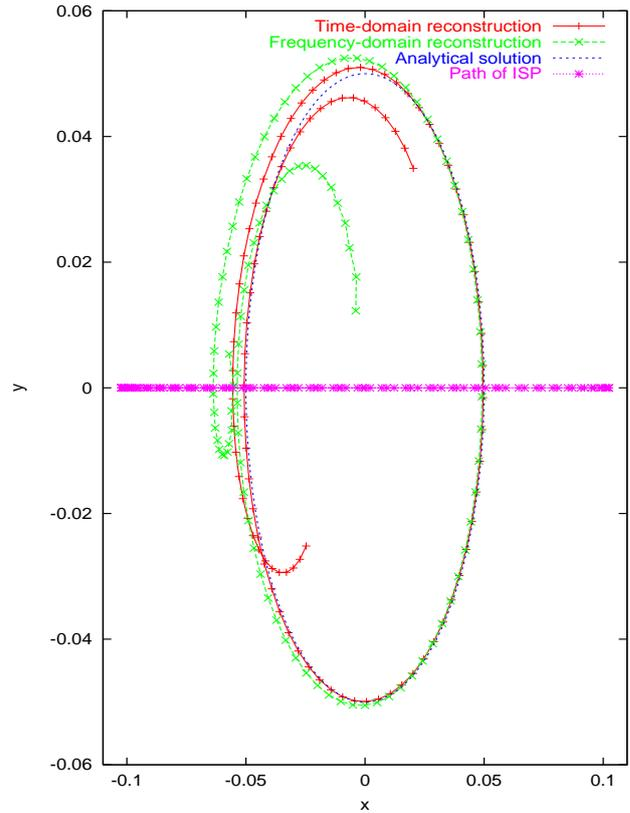
**Fig. 10.** A comparison of the DHT reconstruction algorithms for a rotating Duffing system with  $\epsilon = 0.1$ ,  $\beta = 0$  and  $\omega = 1$ . It is clear that the time-domain algorithm gives better results than the frequency-domain algorithm. The analytical solution is the first-order solution in  $\epsilon$ .
